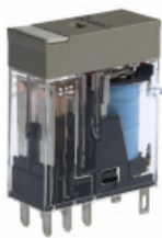
G2R-2-S 12VDC (S) Relay, plug-in, 8-pin, DPDT, 10 A, mech indicator, label facility, 12 VDC
